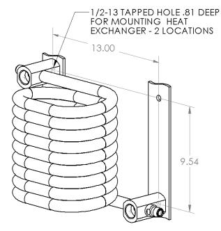
9.54 dimension is mounting height for standard coil length.
